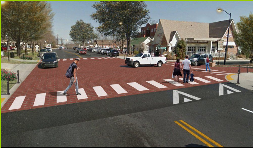
Permanent Raised intersections
