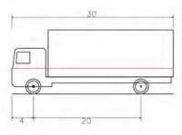
SU — Single Unit Truck Overall Length Overall Width Overall Body Height Min Body Ground Clearance Track Width Lock—to—lock time Curb to Curb Turning Radius
