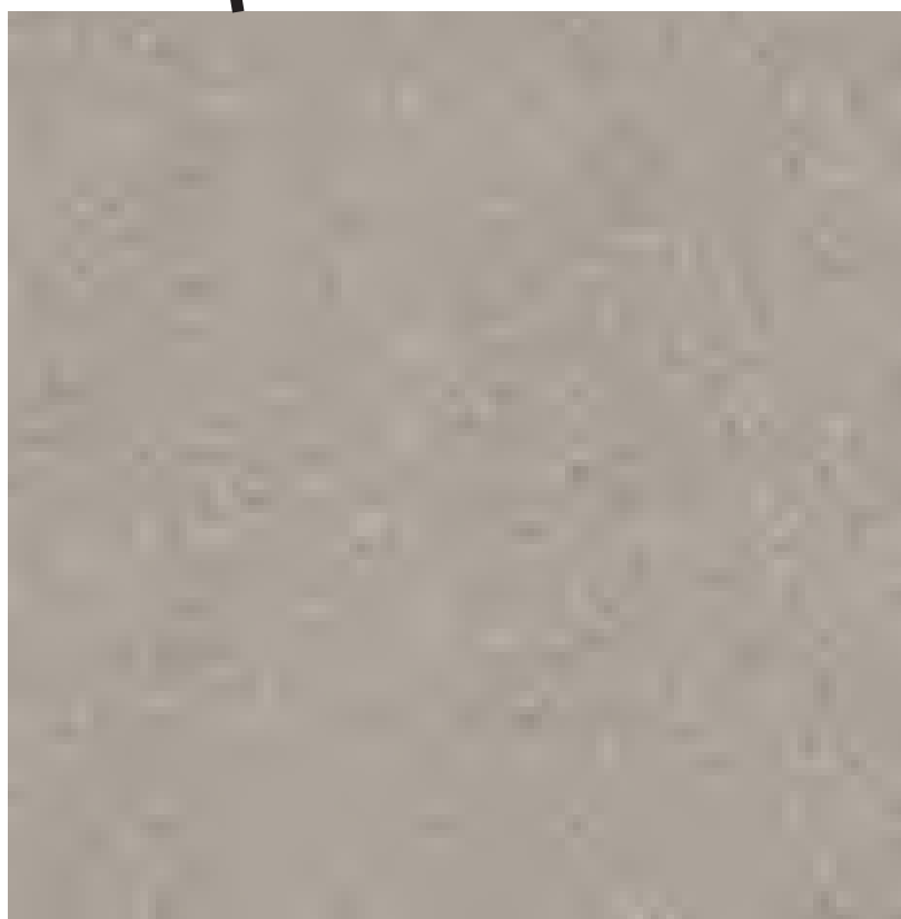
NATURAL CONCRETE FINISH
