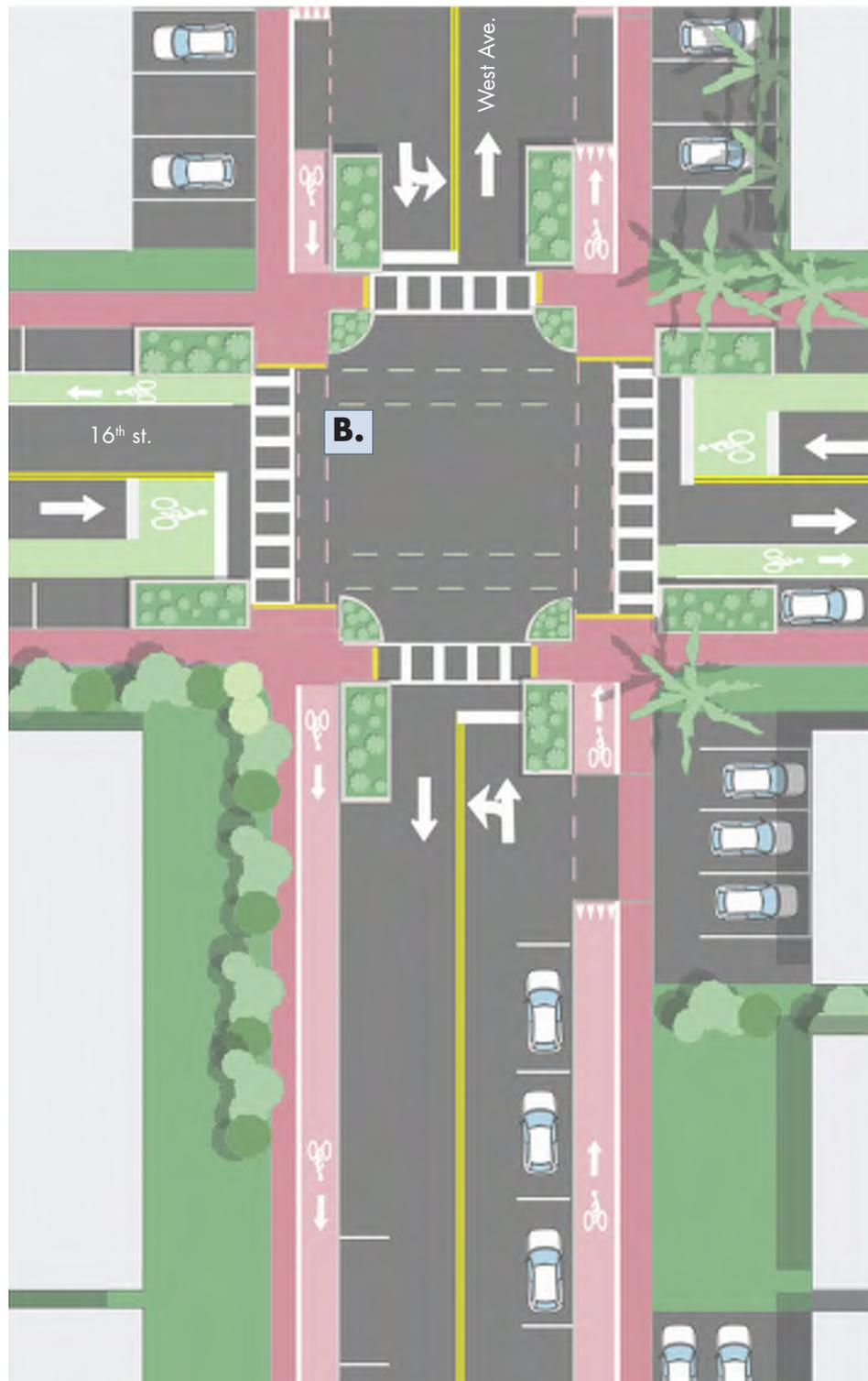
Sidewalk-level bicycle lanes are inherently protected from traffic through vertical separation. In addition, pavement markings or different color treatments help to visually separate pedestrians from bicyclists. In order to protect cyclists from door collisions, this type of facility must accommodate a painted buffer and a 4' lane, or be wide enough ( 5' min.) so as to encourage cyclists to ride in the middle of the lane and avoid conflict.
