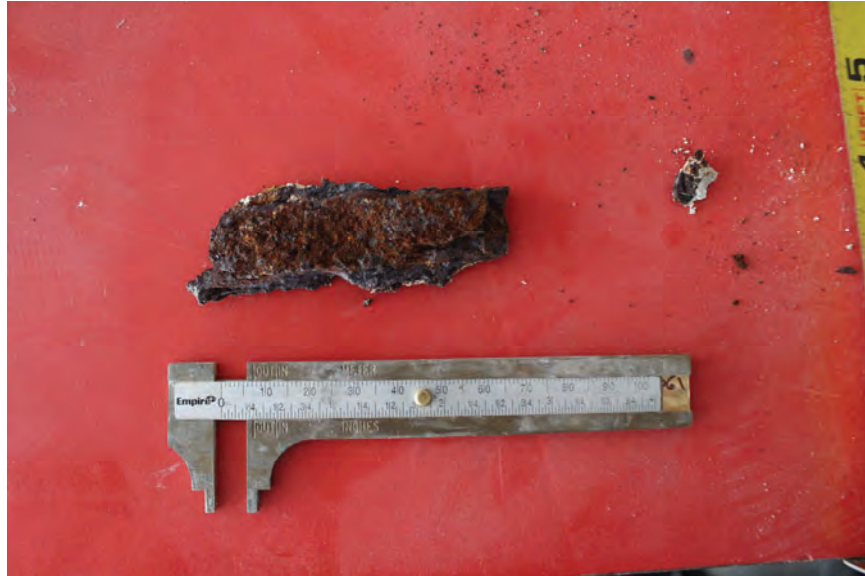
Image 72: Use of caliper to measure thickness of flaked reinforcement steel due to corrosion. This particular photograph exemplifies a typical condition of flakes ranging between 3/16 – 5/16" from #11 bars in Frame Columns.
