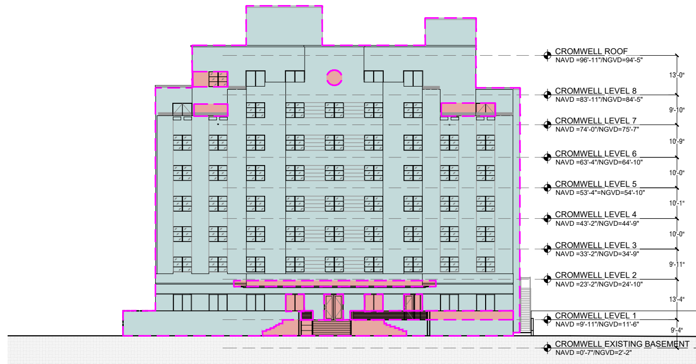
3 DEMOLITION CROMWELL NORTH ELEVATION SCALE: 1/32" = 1'-0"
