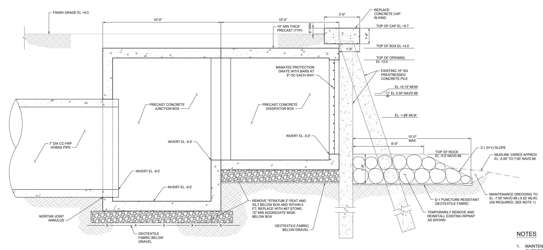
B SECTION - DISSIPATOR BOX AT CENTER LINE OF CULVERT
