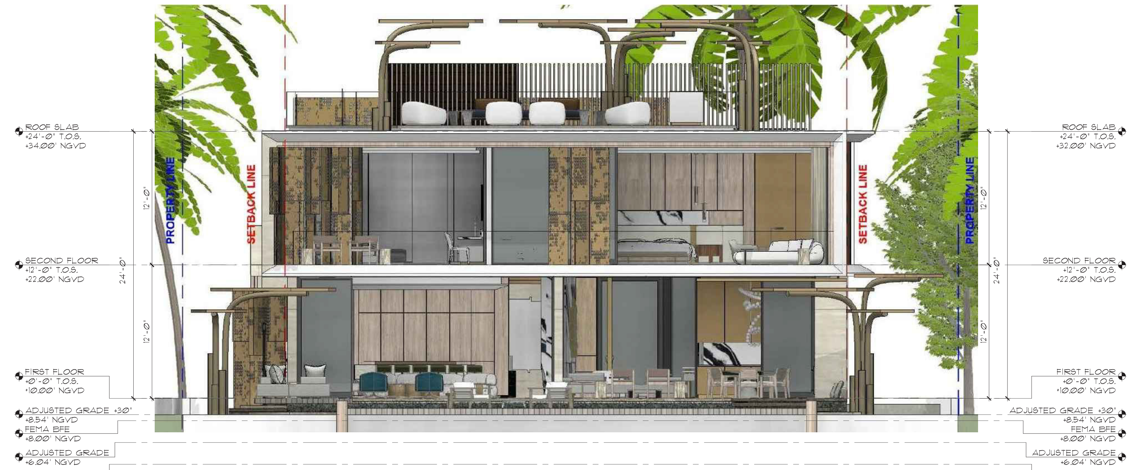
1 A-300 ELEVATIONS REAR (SOUTHEAST) Scale: 3/16" = 1'-0"
