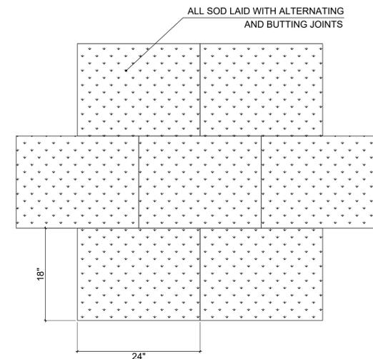
NOTE: PROVIDE 2"-3" OF TOP SOIL FOR FINAL GRADING PRIOR TO LAY DOWN SOD
