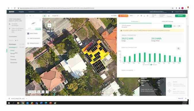
Option#2- Smaller Wattage Panels, using more roof area.
