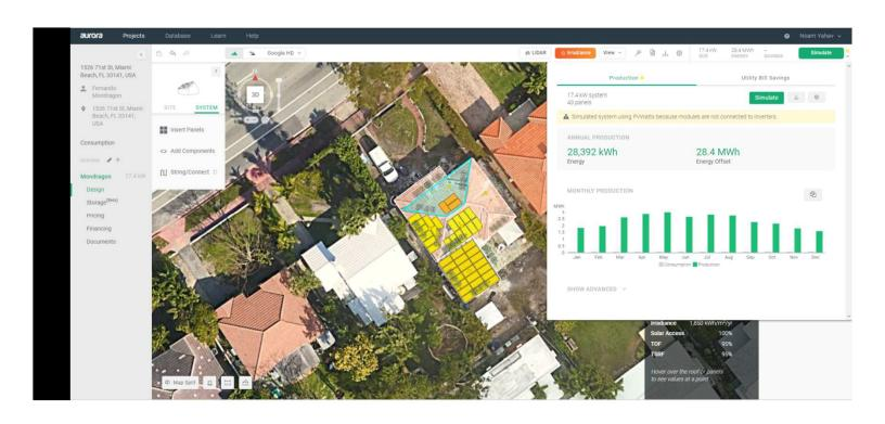
Option #1- Upgraded to 405w panels to reduce the amount of front facing panels
