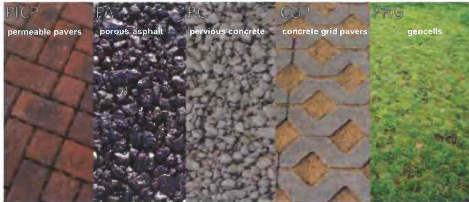
Figure 4. Common Types of Permeable Pavement
