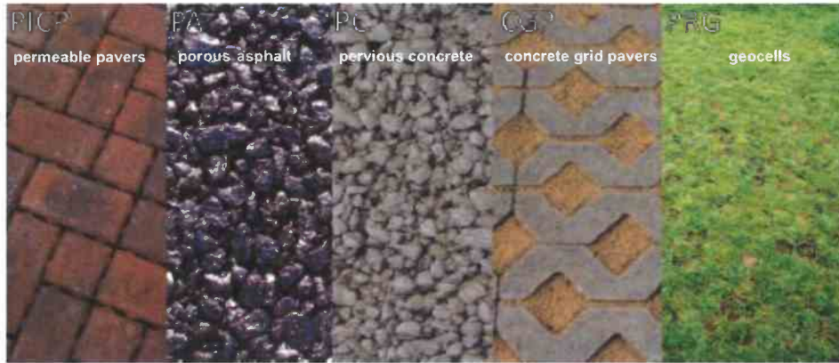
Figure 4. Common Types of Permeable Pavement
