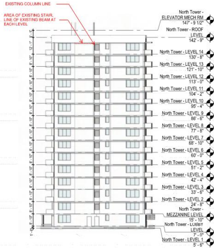
1 PRE-DEMOLITION WING A END ELEVATION SCALE: 1" = 20'-0"
