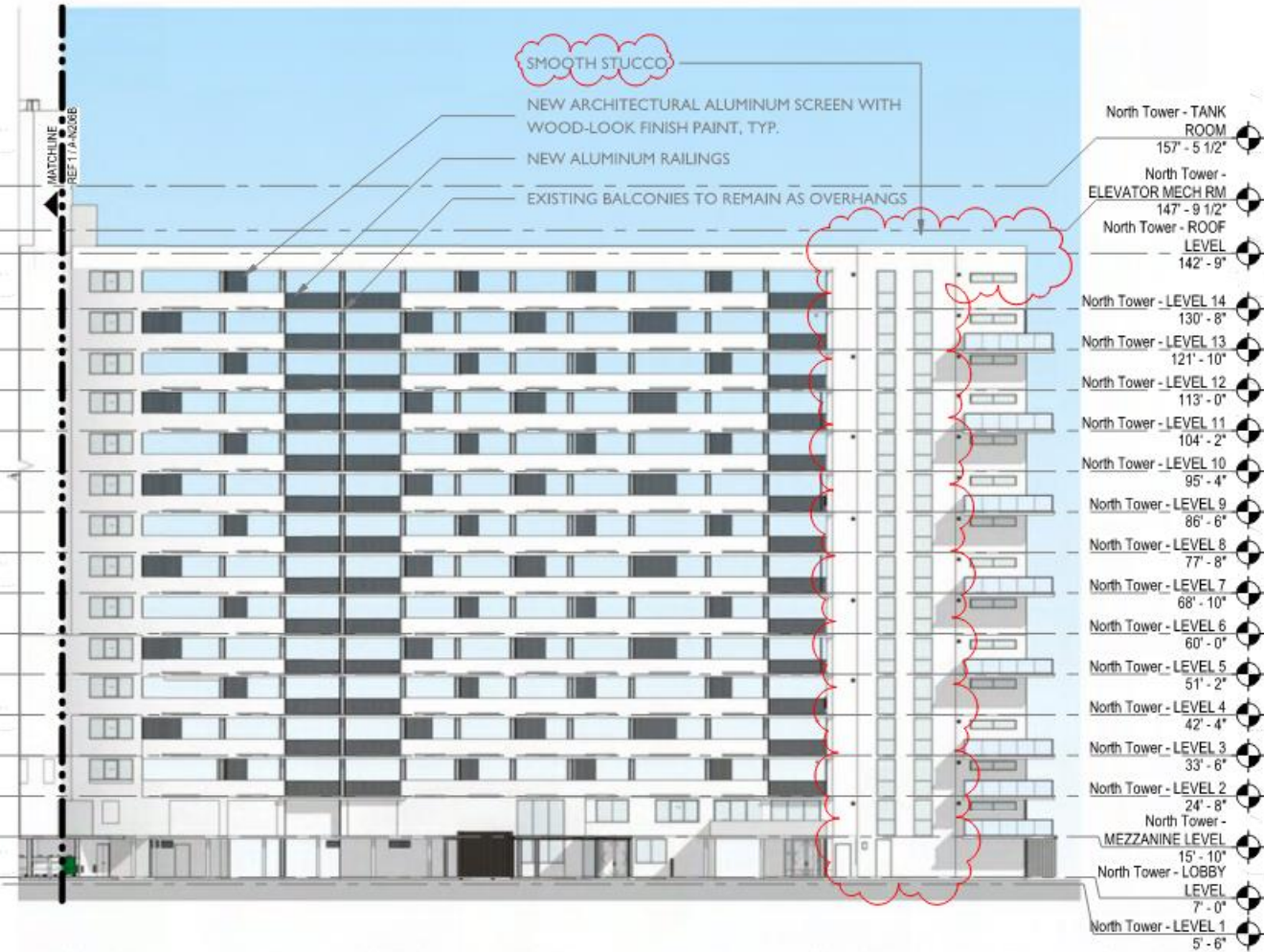
2 North Tower - A Wing East Elevation SCALE: 1" = 20'-0"
