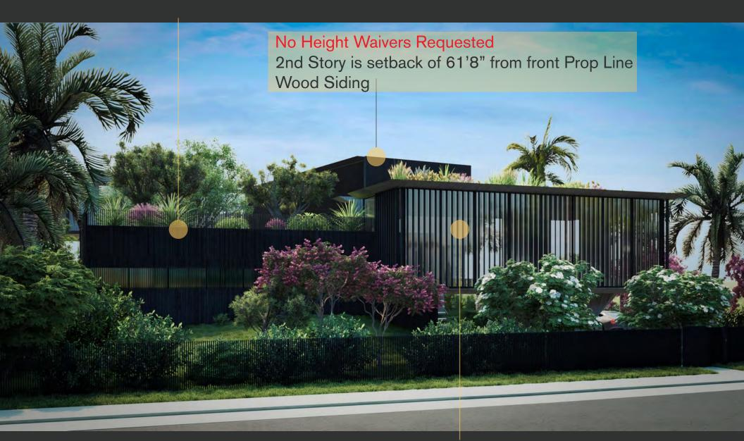
Reduced Height 3'0" Lower, 20'0" Setback from front Prop Line, Wooden Louvers and Extensive Planted Roof
