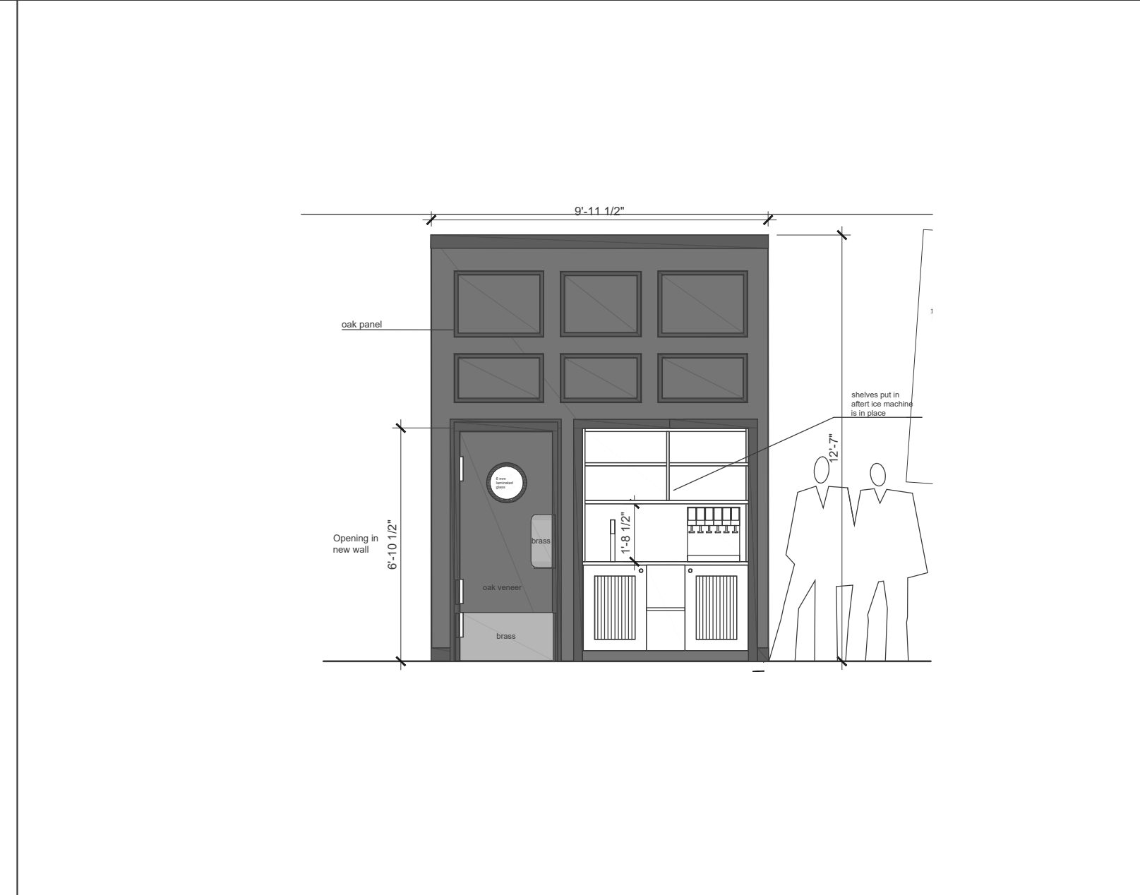
8 BAR STORAGE - SERVING AREA SCALE: 1/4" = 1'-0"
