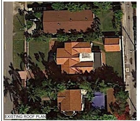
RENOVATION OF HOUSE IN 1990 INCLUDED A COMPLETE CHANGE OF ROOF STRUCTURE. THIS WAS VERIFIED BY OPENING EXISTING OVERHANGS\*. FLAT ROOF SHOWN AT REAR WAS NOT USED IN 1936 AND IS COLLAPSING. (\*SEE ATTACHED PHOTOGRAPHS OF OVERHANG)
