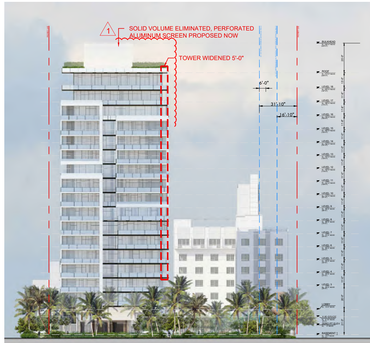
OVERALL EAST ELEVATION - REVISED SCALE: 1"=50'-0"
