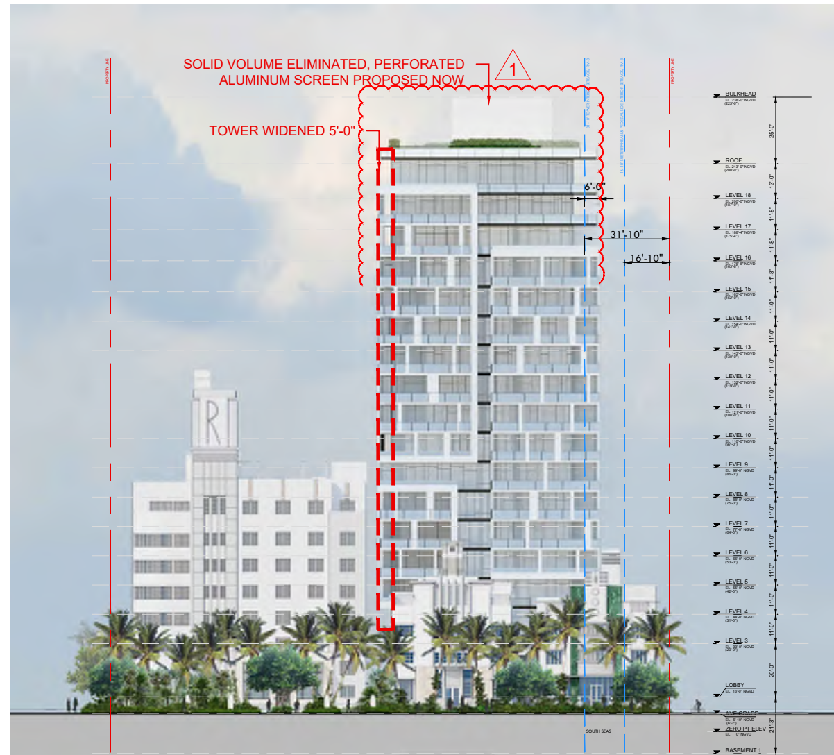
OVERALL WEST ELEVATION - REVISED SCALE: 1"=50'-0"
