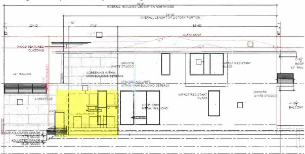
The true "two-story" portions of the residence measure 74'-10" in length. As proposed, the architect has broken up the elevation resulting in an "uninterrupted" span of 55'-10". However, due to the stringent prerequisites of the open space requirements, the side elevation does not satisfy most of the criteria of the regulation. However, the design endeavors the intent of the ordinance since the designated open space successfully breaks up the massing of the two-story elevation.
