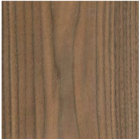
WD1 ALUMINUM PANEL CLADDING- WOOD FINISH
