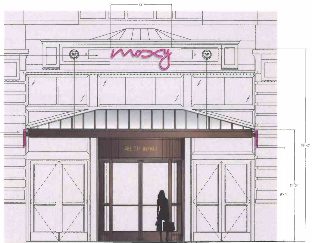
2 BUILDING ID B1 & B1.1 FRONT ELEVATION - 1/10 SCALE SUBSTRATE 3" DEEP C CHANNEL, L11 FLRS WITH INTERNAL 15mm neop. SEE DRAWINGS X2 & X3 FOR DETAILS
