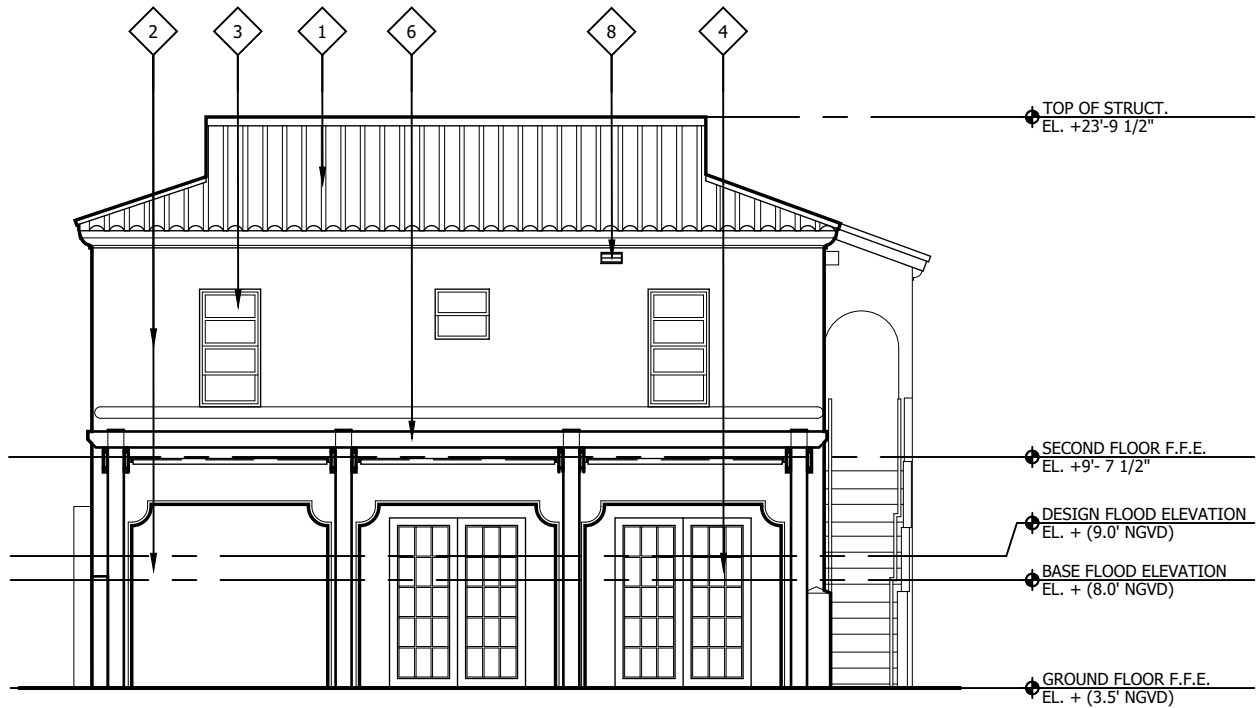
D EXISTING BUILDING B: NORTH ELEVATION SCALE: 1/8"=1'-0"
