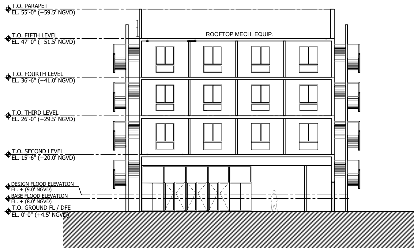
1 BUILDING SECTION 1 SCALE: 1/16"=1'-0"
