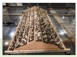
determine the amount of energy that is reduced by the breakwater. To date, we have run over 50 experiments to test the reduction in wave energy under different wind and wave conditions, and have found that we can make engineered structures *more* effective at protecting our coasts **by at least 15%** by adding corals to their surface!
