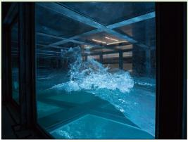
wave tank capable of simulating up to a category 5 hurricane. This facility allows us to investigate at a fine scale the physical dynamics of waves as they interact with corals and model breakwater structures. As waves travel from one end of the tank to the other, they carry energy towards the model shoreline. By measuring the wave height before and after the breakwater model, we can
