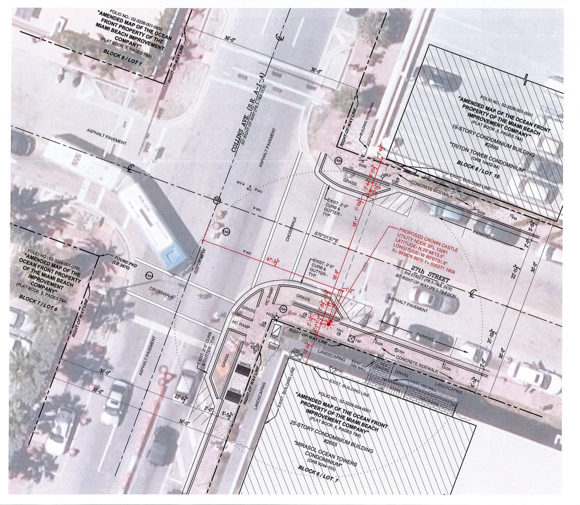
**LEGEND** EXISTING DRAINAGE MANHOLE (FDOT WHERE SHOWN) EXISTING ELECTRIC MANHOLE ₹8X EXISTING ELECTRIC BOX FAH EXIST. FIBER OPTIC HANDHOLE EXIST. FIRE DEPT. CONNECTION FH EXISTING FIRE HYDRANT EXISTING ELECTRIC MANHOLE ☐ PM EXISTING PARKING METER PEDS EXIST. PEDESTRIAN SIGNAL EXISTING SIGN 0 EXISTING STREET LIGHT MH EXISTING TELEPHONE MANHOLE TD EXISTING TRENCH DRAIN TRH EXISTING TRAFFIC HANDHOLE EXIST. TRAFFIC SIGNAL POLE EXISTING WATER VALVE
