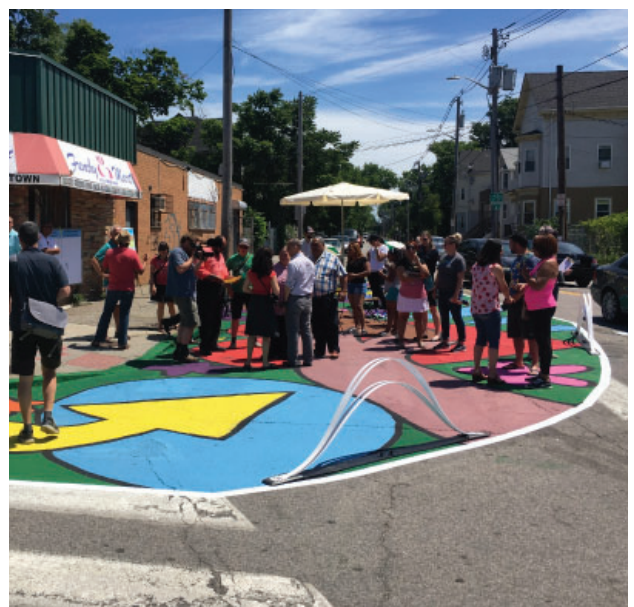
Another large curb extension at Broad St. and Public St. corrected the geometry of the intersection, and created space for people to gather.
