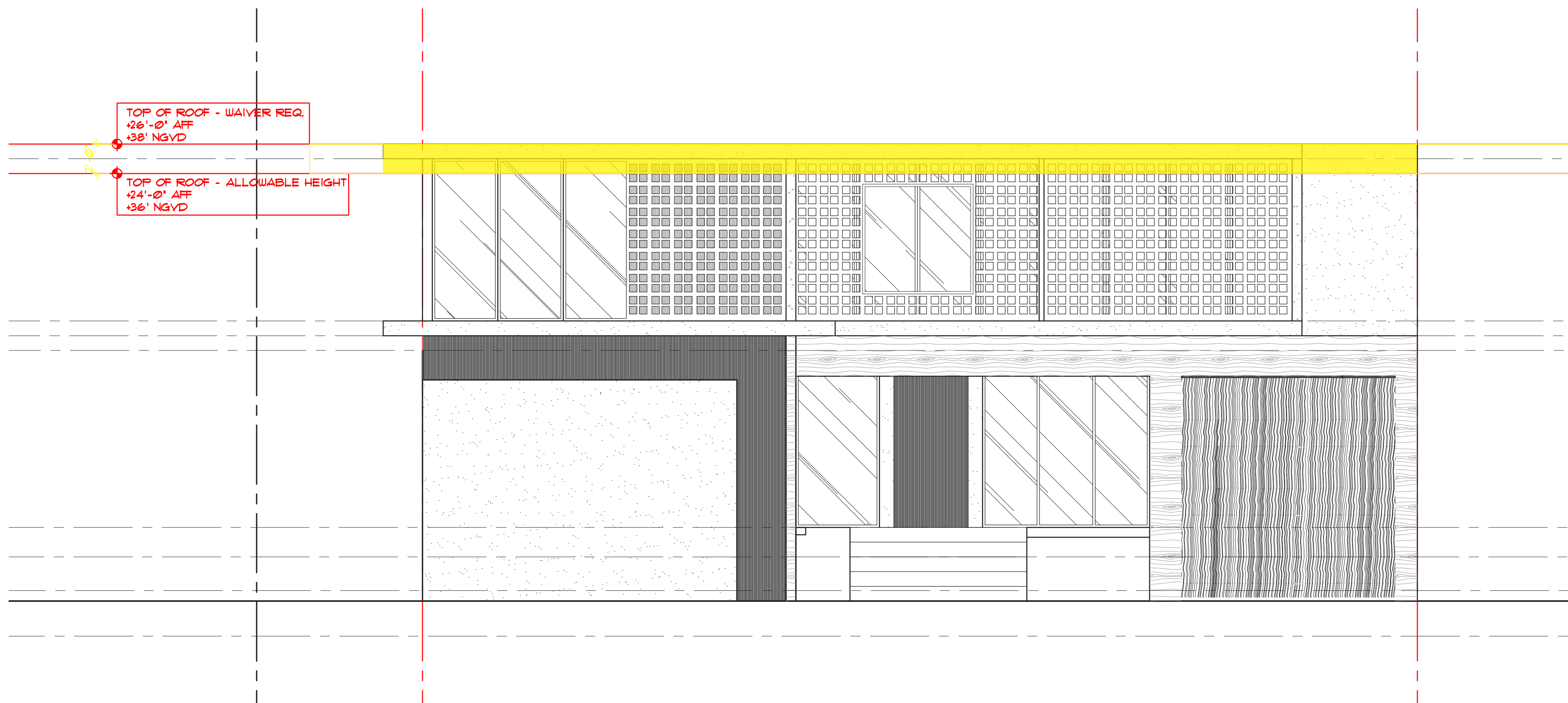
BACK ELEVATION - WAIVER DIAGRAM SCALE: 3/16"=1'-0"
